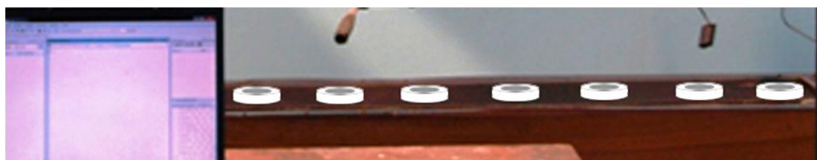
Fig 5.2: A mechanical system of grooves on conveyor belt to hold and orient apples.
