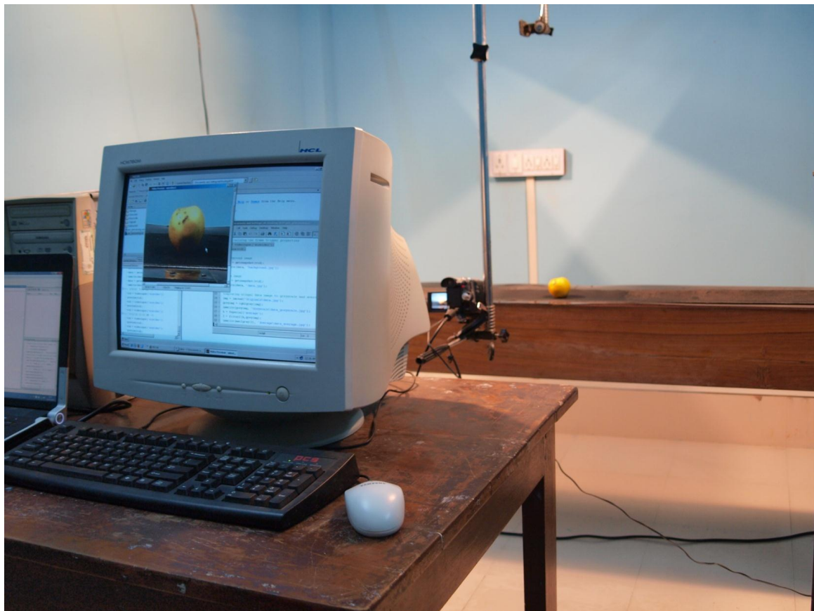
Fig 4.4: Capturing live data of the apple using IEEE connector with MATLAB
